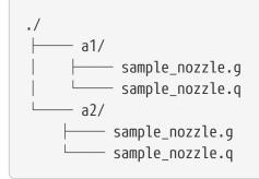
In other words, two case folders, a1 and a2, each containing a pair of PLOT3D files (the .g and .q files). You will create a sample\_nozzle.mcr file, a Tecplot macro that loads the PLOT3D files, and deposit a copy in each case folder. The resulting structure will look like this:
