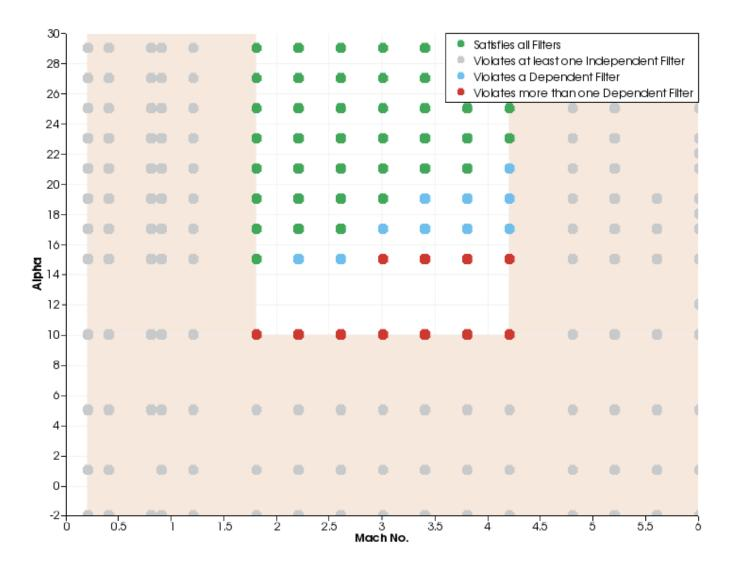
In this example, the filters have been set to exclude cases by Mach No. and Alpha (the shaded area, with the individual cases shown in gray because they also violate a filter on an independent variable) and also to exclude certain other cases by their lift and drag coefficients. These cases are displayed in blue (for cases that only violate one of the lift and drag constraints) or red (for cases that violate both the lift and drag constraints).
