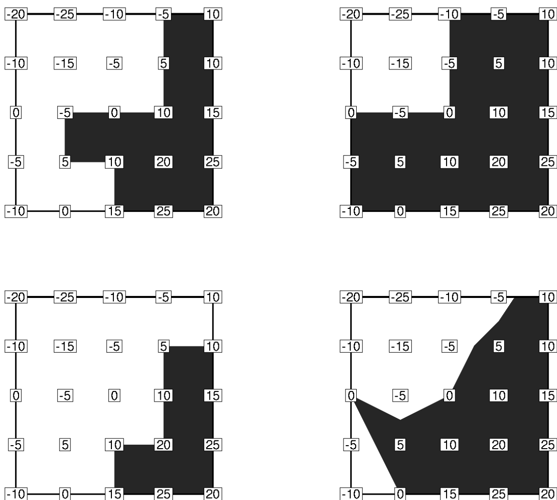
Figure 55. The effects of the different value blanking options in field plots for a constraint where a variable is less than or equal to zero. The dark shading indicates the areas that are not blanked. Clockwise from upper left: Blank cell when primary value is blanked. Blank cell when all corners are blanked. Trim cells along mathematical constraint boundary. Blank cell when any corner is blanked.
