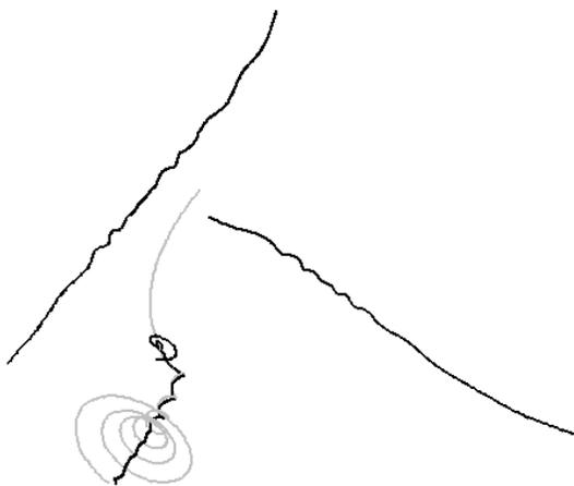
Figure 6e Result of FAST vortex core finder on data set 3. Note that a streamline has also been spawned here to indicate that the twist at the top of the middle curve is actually outside the vortex.
