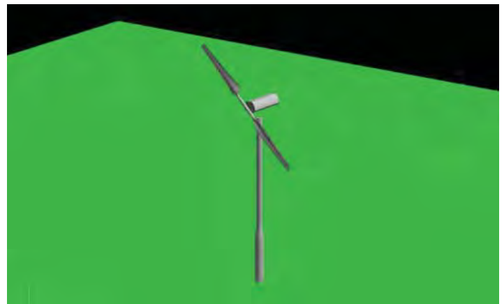
Figure 2: Modeled NREL 10 m wind turbine geometry (solid surfaces)
